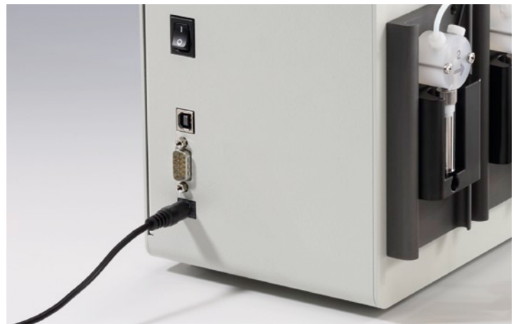
Sirius L supports both USB and RS-232 data ports
